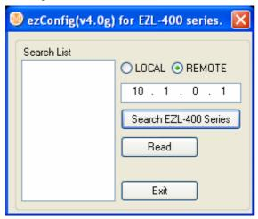
For the REMOTE SEARCH, user should select the [REMOTE] radio button in the initial window and input an IP address and press [Search EZL-400 Series], then the ezefgmp searches EZL-400S with the IP address.
