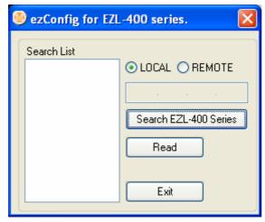
The LOCAL SEARCH method use UDP local broadcast with MAC address. So its benefit is that user can search EZL-400S although the user doesn't know the IP address of EZL-400S. For LOCAL SEARCH, user should select [LOCAL] radio button and press [Search EZL-400 Series]. Then the ezcfgmp searches all EZL-400Ses in the local network. The found EZL-400Ses appear in the [Search List] window in form of its MAC address.
